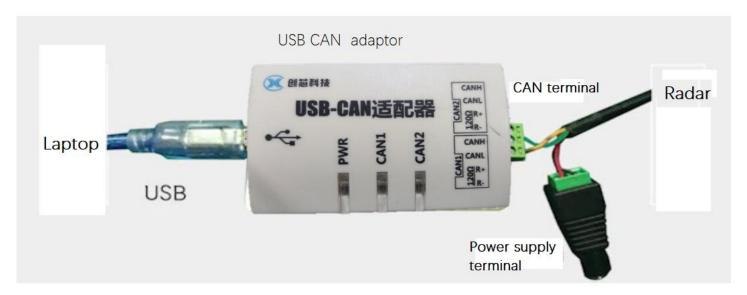
4. Connect the USB interface of the USB CAN box(adaptor) to the laptop and open the test software.
