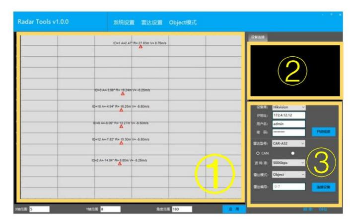
Area ① is the radar coordinate map, showing the radar detection results; Area ② is the camera display for comparison and recording test; Area ③ is the radar setting function interface. Click "connect equipment" button to connect the radar.
