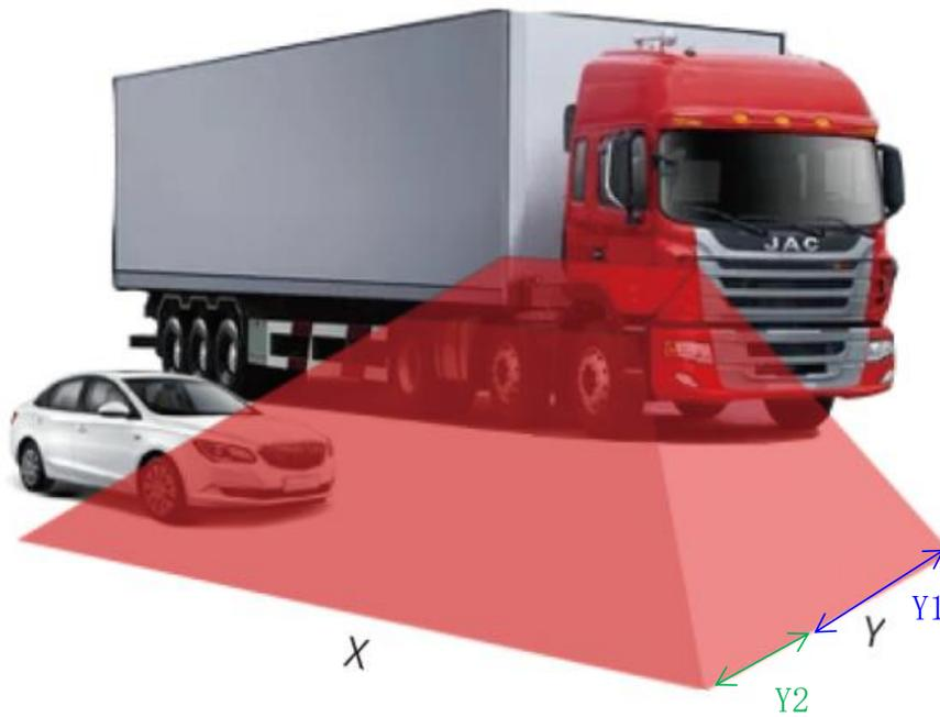
Figure6.1 Alarm range diagram
