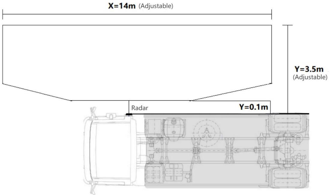
Figure5.1 Top view of radar detection area
