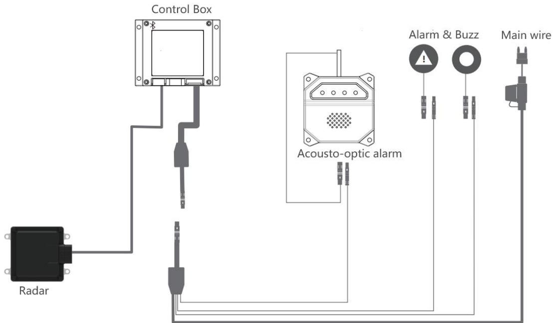
Figure4.1 Wiring diagram of radar system
