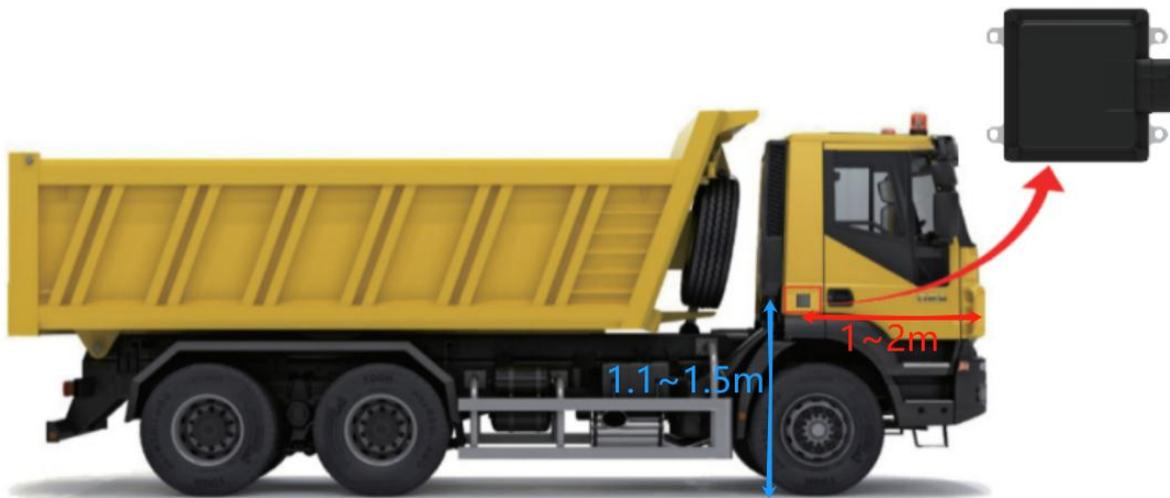
Figure5.2 Schematic diagram of radar installation
