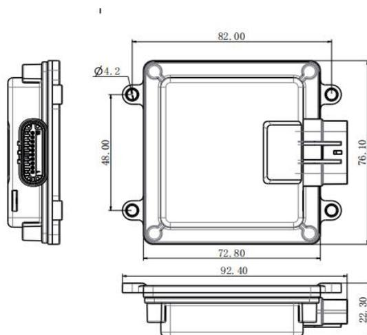
Figure 2.1 Dimension drawing of radar
